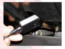
6. The USB cable can easily be hidden under the dash for later data retrieval via a laptop computer or the entire Trackstick Pro can be removed during download if the vehicle layout permits.
